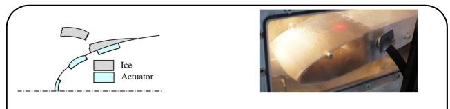
Diagram of operation of an electromechanical system (de-icing mode). Ice forms on the protected area. An actuator deforms the surface locally, inducing the expulsion of ice.
